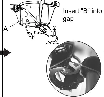
Align bolt to groove
