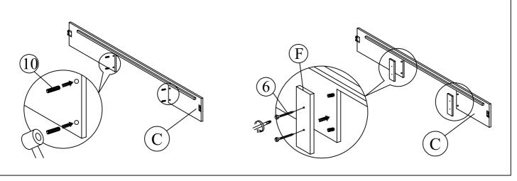
Step 3 : Attach side rail (C) to headboard (A) and footboard (B) by pushing the bracket down to fit it.
