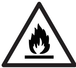
Please keep the product far away fire source during using, service and disposal. There are flammable materials at the back of the appliance. Please according to local regulations regarding disposal of the appliance for its flammable blowing gas, Before you scrap the appliance, please take off the doors to prevent children trapped.
