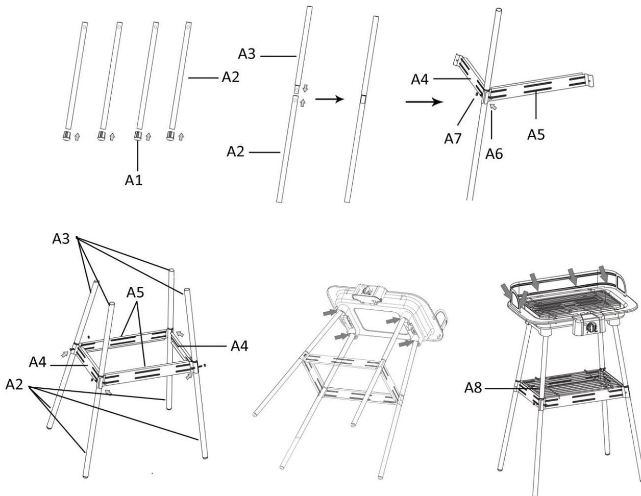
1. Insert 4 fittings (A1) into the end of the long pipe openings.
