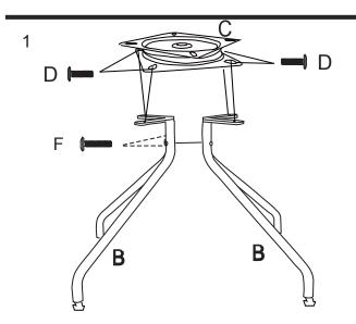
Attach the leg B with screws F,then C with screws D as show.
