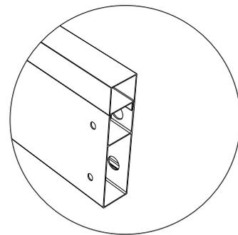
Check size. Use a  $\varnothing 12\text{mm}$  drill bit to drill holes on the position where to fix the steel plate, then fix steel plate with **TO**. Use a M17 wrench to fasten the **TO**.
