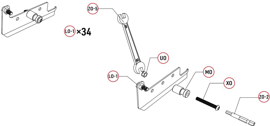
Use **ZO-5** to fix the **UO** and complete the assembly of the **LO-1**.
