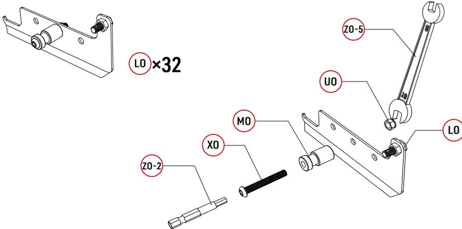
Use **ZO-5** to fix the **UO** and complete the assembly of the **LO**.
