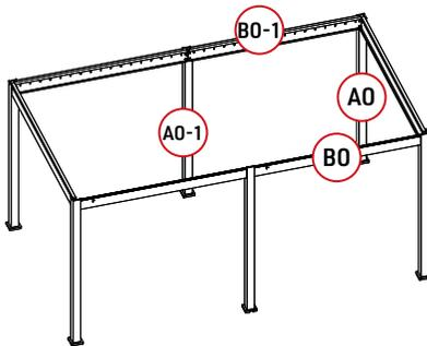
1. Lay the column and beam flat, and put **B0-1** into the groove of the completed column **A0**.
