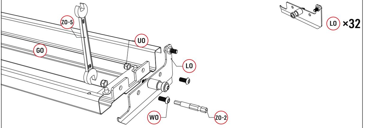
Install the connecting pieces at both ends of the louver.
