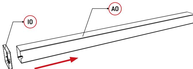
1. Place the **I0** into the **A0**, making sure that the notch around the column **I0** is aligned with the drain outlet at the bottom of the **A0** column, and place it into the column.
