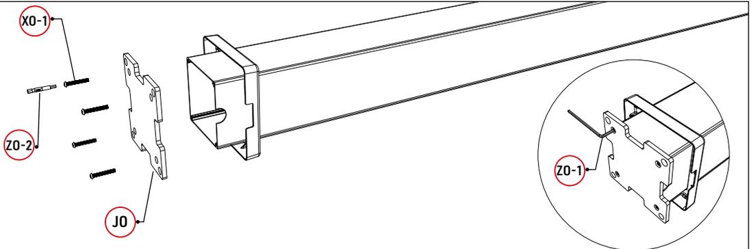
2. Use **X0-1** to connect the **J0** base plate to the bottom of the column, and use the hexagonal wrench **Z0-1** to tighten the screws manually.
