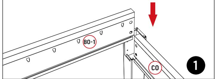
2. Connect **B0-1** with **A0** using **Q0**. Use hex wrench **Z0-3** to tighten manually.
