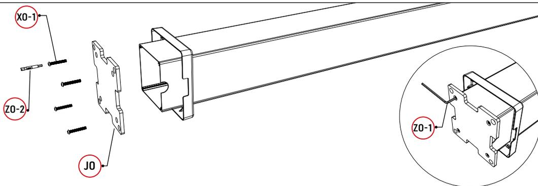
2. Use **X0-1** to connect the **J0** base plate to the bottom of the column, and use the hexagonal wrench **Z0-1** to tighten the screws manually.
