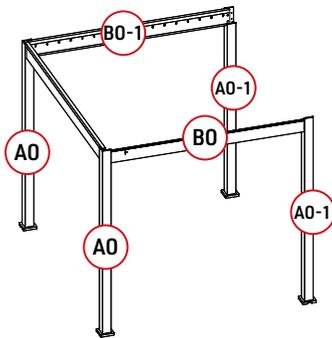
1. Lay the column and beam flat, and put **BO-1** into the groove of the completed column **AO**.
