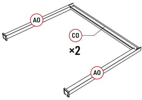
1. Lay the column and beam flat, and put **CO** into the groove of the completed column **AO**.
