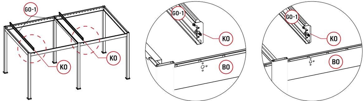
Place the **KO** end into the cavity of the **BO** as shown in the picture.
