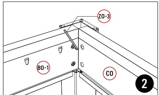
3. Connect **B0-1** with **A0-1** using **Q0**. Use hex wrench **Z0-3** to tighten manually. **B0** is installed in the same way
