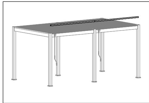
Cover the holes on the beam by using **RO**.
