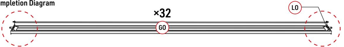
Install the connecting pieces at both ends of the louver.
