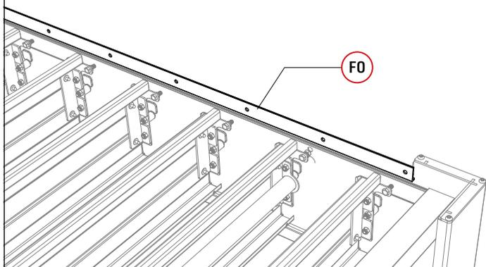
Use **U0** at both ends of spindle **G0-1** to fix both ends of **F0**.
