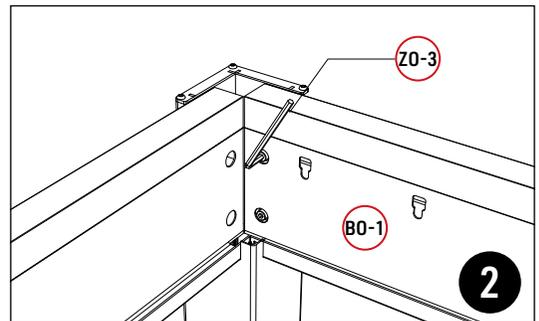
3. Connect **BO-1** with **AO-1** using **QO**. Use hex wrench **ZO-3** to tighten manually. **BO** is installed in the same way
