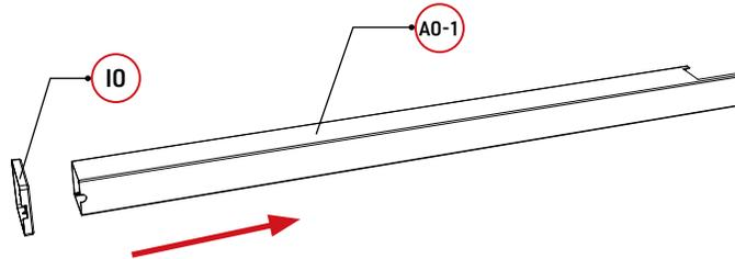
1. Place the **I0** into the **A0-1**, making sure that the notch around the column **I0** is aligned with the drain outlet at the bottom of the **A0-1** column, and place it into the column.
