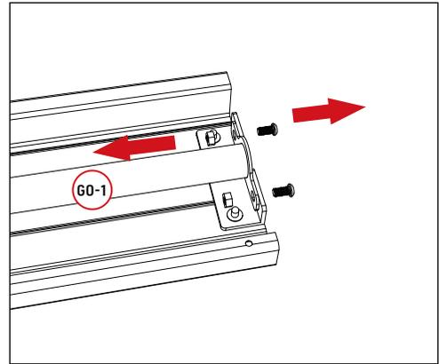
Install the connecting pieces at both ends of the louver.
