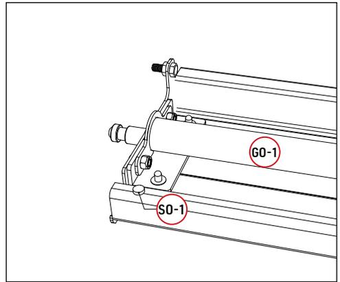
Install **S0-1** on both ends of the louver
