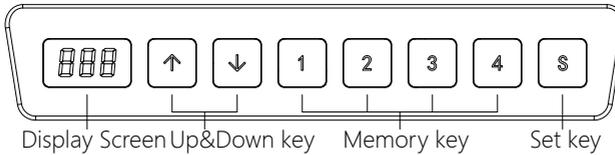
The whole handset surface is a button panel. If there is no press within 30 seconds, the screen is locked and 1/2/3/4/S keys are locked correspondingly, you should press Up or Down key first, it can be used when the display screen light up.
