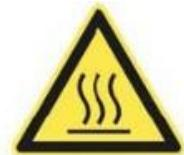
Please do not touch surface while in use. The temperature of accessible surfaces may be high when the appliance is operating.
