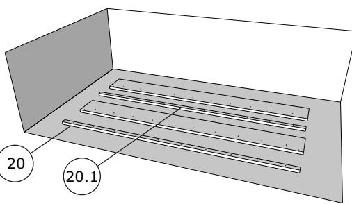
Put the left panel of the bed on ground facing frontside and make sure that there is nothing bellow the panel
