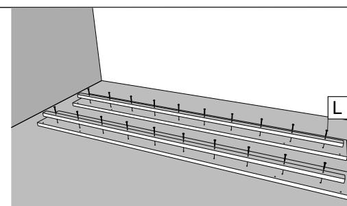
Gently apply pressure on the surface of the panels and secure them with screws.
