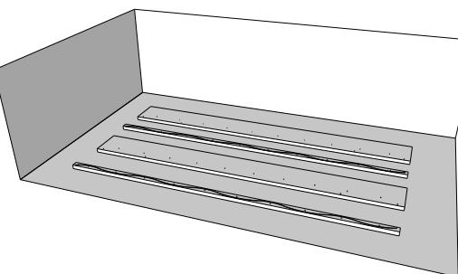
Make sure that all panels that you need to apply glue to are clean from dust,dirt and oil and then apply glue on them.
