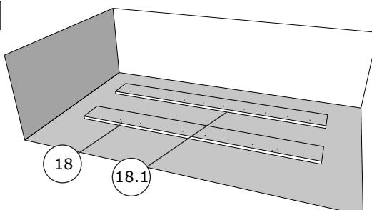
Put the side panels of the bed on ground facing backside and make sure that there is nothing bellow the panel
